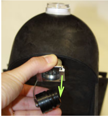
Figure 2-8 Preparing the LaserFlow connector receptacle
