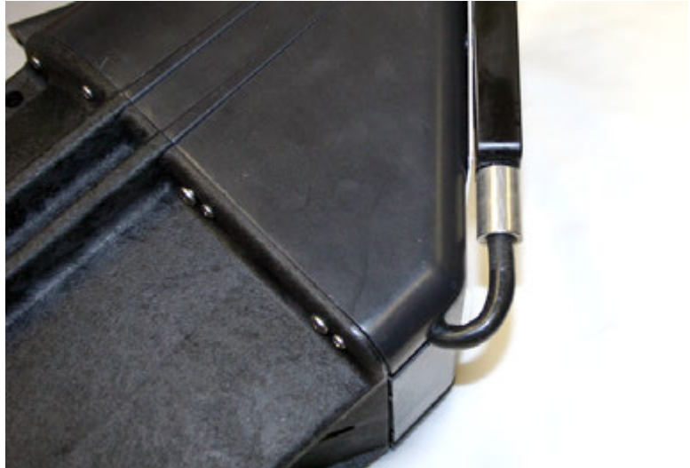
Figure 5-7 Reassembling the LaserFlow w/ AV sensor installed
