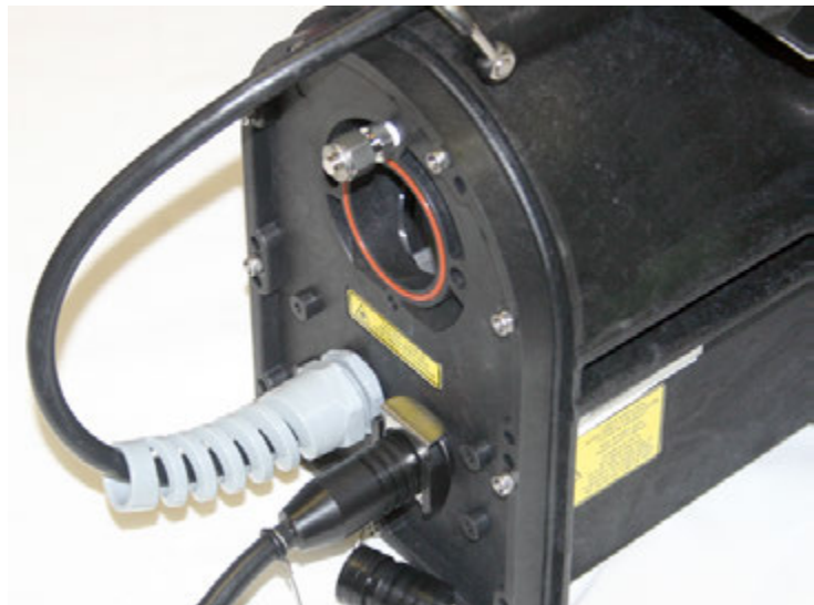
Figure 5-6 Connecting the 350 AV sensor to the LaserFlow
